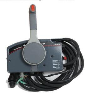
Side Mount Control Boxes can be tailored to your needs. Standard features include a fast idle lever for easy Warm-ups, a Key-type ignition Switch, and an emergency stop switch. No Trim and tilt switch. 7 Pins wire harness included.
