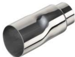
YWX-107 | Length:147mm Inlet: ø 50.8mm Outlet: ø 77x48.5mm Angle:30°
