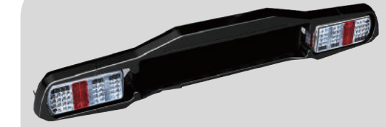
CF-006 Size: 1070 x 130 x 60 mm Material: PP
