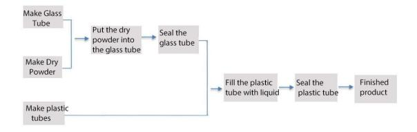
**Special instructions:** Our factory has a special workshop for making glass tubes. A series of processes, from pipe making to batching and packaging, are completed by the factory itself. There is no need for external procurement, which can save costs and enhance quality control. Other manufacturers do not have glass tube production workshops, so
