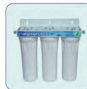
UMK-PR303 Triple filtration PP+GAC+CTO Inlet pressure: 8-125 PSI./ 0.6-8.8 kg/cm 2 With a wrench,faucet and other small accessories.
