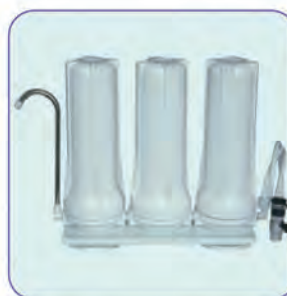
UMK-TR203 Triple filtration PP+GAC+CTO Inlet pressure: 8-125 PSI. 0.6-8.8 kg/cm 2 With a wrench,contains a diverter and a faucet.
