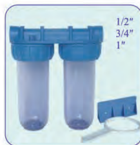
UMK-BR10B3 Inlet pressure: 8-125 PSI. 0.6-8.8 kg/cm 2 With plastic bracket, wrench, brass port.
