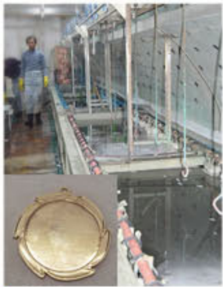
03 Plating pyrophosphate copper
