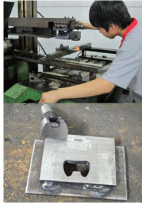
07 Making the die cut mould
