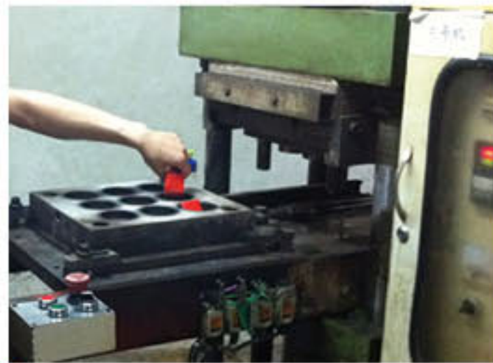
06 Put material inside mould
