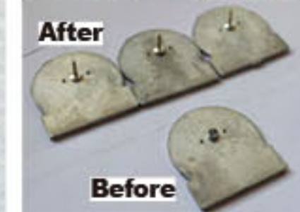
11 Riveting butterfly clutch *if necessary
