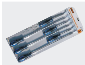
Handle: hard pp core, soft TPE cover with round cross-section, Blade: round, satin chrome plated, carbon steel, hardness 41HRc Function: Pull round plastic parts on the body
