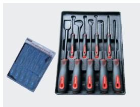
Handle: hard pp core, soft TPE cover with round cross-section. Blade: round, black finish plated, Cr-V steel.
