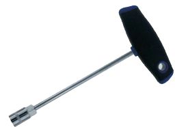
Handle: 2-component, T-shaped hard PP cover, soft TPR cover. Blade: hexagonal, two-sided, black finish, surface point tips.
