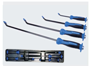
Handle: hard pp core, soft TPE cover with round cross-section, Blade: square, satin chrome plated, carbon steel, hardness 40HRc Function: after body percussion
