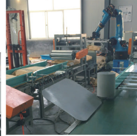
▼ 1 robot works with 2 assembly to do palletizing
