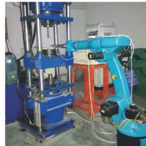
▲ Punching machine material loading and unloading
