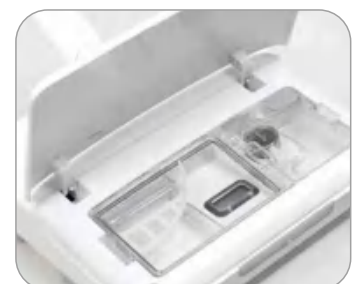
Outlay Water Tank and Dust Box
