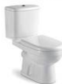
1560-2967 Washdown two-piece toilet Size: 710x410x750mm S-trap: 250mm Roughing-in P-trap: 180mm Roughing-in
