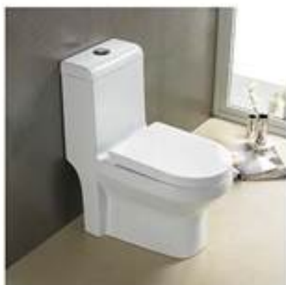
1512-2806-S Siphonic one-piece toilet Size: 710x380x800mm S-trap: 300/400mm Roughing-in
