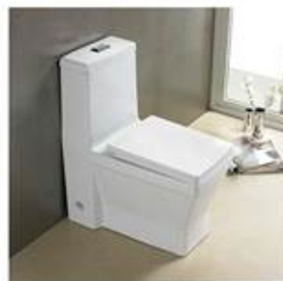
1515-2829 Siphonic one-piece toilet Size: 660x350x800mm S-trap: 300/400mm Roughing-in
