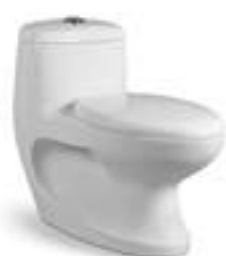
1547-2930 Washdown one-piece toilet Size: 700x380x660mm S-trap: 100/230/300mm Roughing-in P-trap: 180mm Roughing-in
