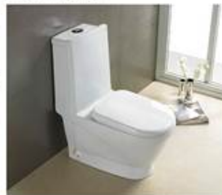
1500-2869 Washdown one-piece toilet Size: 750x400x800mm S-trap: 250/300mm Roughing-in P-trap: 180mm Roughing-in
