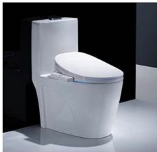
1599-1801 Intelligent seat cover Size 505x375x135mm Washdown one-piece toilet Size 660x400x780mm S-trap:250/300/400mm Roughing-in P-trap:150mm Roughing-in
