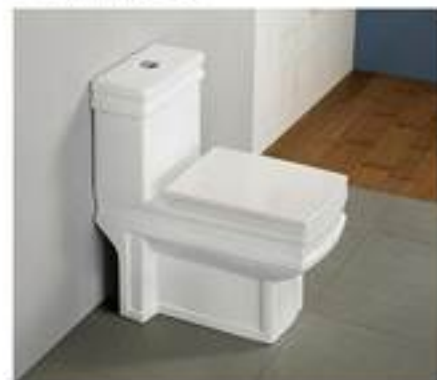
1498-1128 Washdown one-piece toilet Size: 720x350x770mm S-trap: 250/300mm Roughing-in P-trap: 180mm Roughing-in
